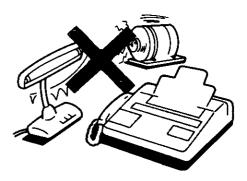
The unit and the cassette tape should be kept free from dust, moisture, high temperature and vibration.
